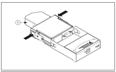
1 High Voltage Screw Terminal Backshell
